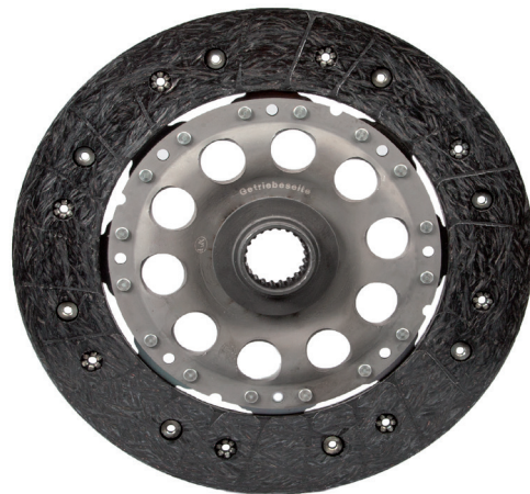
Fig. 2: Original equipment clutch disc (diameter 240mm)
